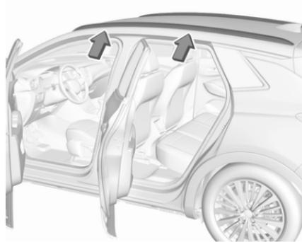
Fasten the roof rack in the roof railing above the mounting points located in each door frame of the vehicle body.
