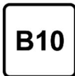
Diesel fuel that meets standard EN16734 mixed with a biofuel that meets standard EN14214 (possibly containing up to 10% Fatty Acid Methyl Ester).
