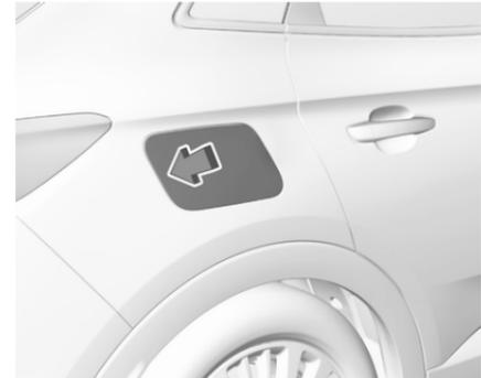
The fuel filler flap can only be opened if the vehicle is unlocked. Open the fuel filler flap by pushing the flap.
