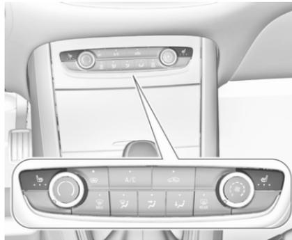
Adjust heating to the desired intensity by pressing
