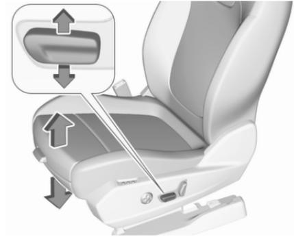
Move switch upwards / downwards.
