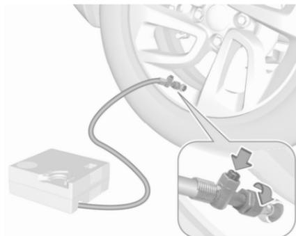
18. Continue driving immediately so that sealant is evenly distributed in the tyre. After driving approx. 3 miles but no more than ten minutes, stop and check tyre pressure. Screw compressor air hose directly onto tyre valve when doing this. Fill tyre as described
