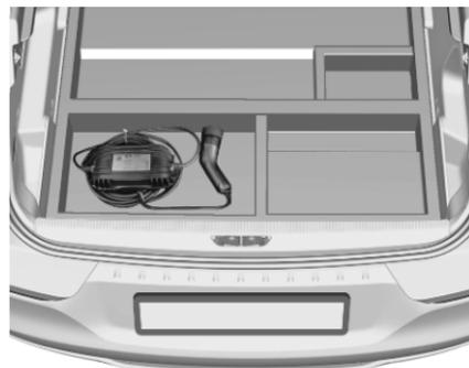
3. If necessary, take the charging cable out of the load compartment.
