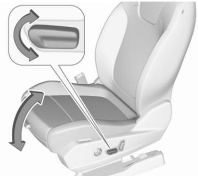
Move front of switch upwards / downwards.
