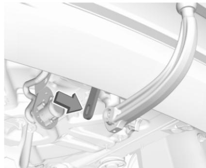
Attach breakaway stopping cable to eye.
