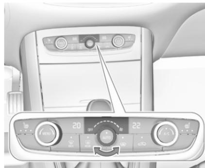
Different pre-set fan speeds can be set by turning the rotary knob.
