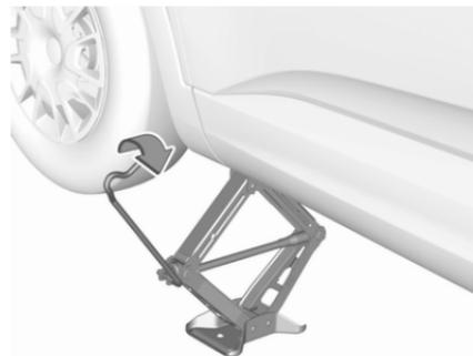
With the jack correctly aligned rotate wheel wrench until wheel is clear of the ground.
