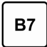
Diesel fuel that meets standard EN590 mixed with a biofuel that meets standard EN14214 (possibly containing up to 7% Fatty Acid Methyl Ester).
