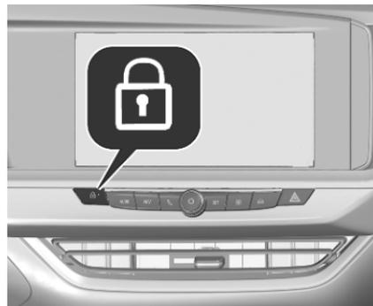
This function can be activated or deactivated at any time. With the ignition on, press
