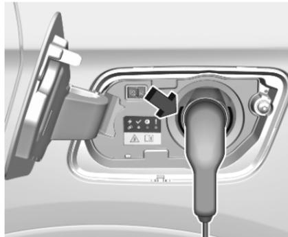
The start of charging is indicated by the green flashing of the status indicator at the charging port and at the control box of the charging cable if available.
