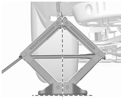
4. Set the jack to the necessary height. Position it directly below the jacking point in a manner that prevents it from slipping.
