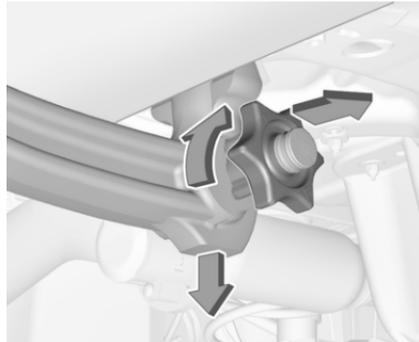
Open the protective flap and turn the key to position
