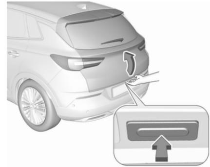
After unlocking, press the tailgate button and open the tailgate.
