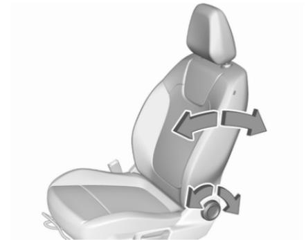
Turn handwheel. Do not lean on backrest when adjusting.
