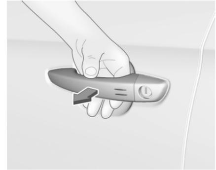
Pass a hand behind the door handle of a front door to unlock the vehicle or press the tailgate button.
