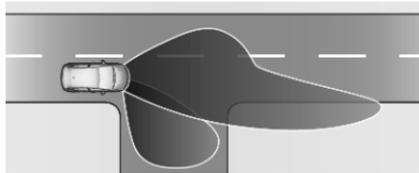
Activated at a speed of up to approx. 25 mph when turning off. Depending on the steering wheel angle and the turn lights, a particular LED light function is triggered which illuminates the direction of travel.
