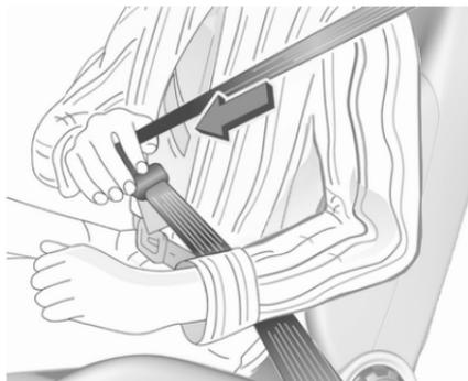
Withdraw the seat belt from the retractor, guide it untwisted across the body and insert the latch plate into the buckle. Make sure the belt fits tightly to the body while driving.
