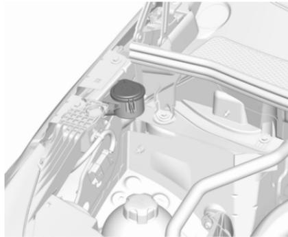
Fill with clean water mixed with a suitable quantity of approved windscreen washer fluid which contains antifreeze.
