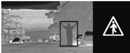
If a collision is imminent, the object detected is displayed in a red frame and an alert symbol is triggered.
