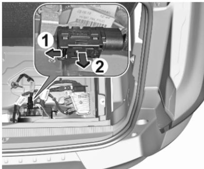
7. Hybrid vehicle: Push (1) the unlock lever and remove (2) the lead from the connection pin.
