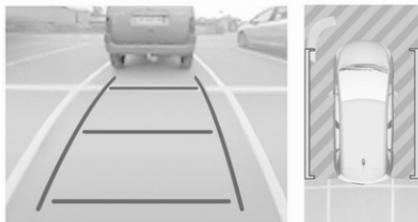
The screen in the Info Display is divided into two parts. On the right there is a view from above the vehicle and on the left there is the view from the rear or the front displayed. The parking sensors complete the information on the view from above the vehicle.
