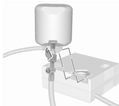
Type B: Screw the compressor air hose to the connection on the sealant bottle.
