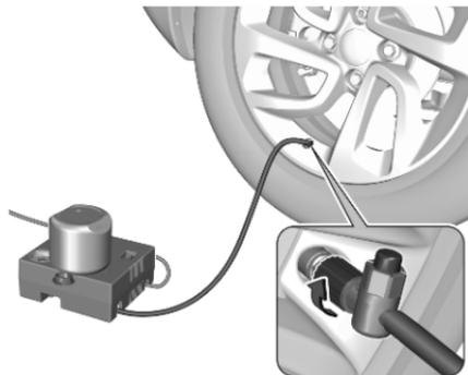
9. Screw the filler hose to the tyre valve.
