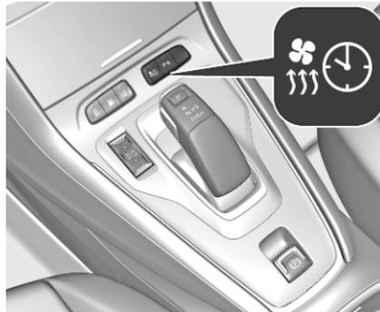
The operating status of the temperature preconditioning is shown by a LED.
