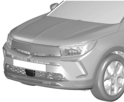
The radar unit is located in the middle of the front bumper.
