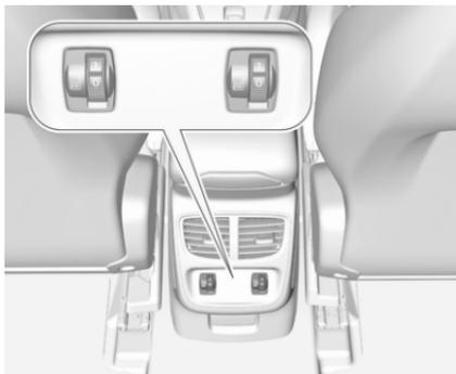
Adjust the seat heating by turning the thumb wheel
