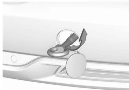
Screw in the towing eye as far as it will go until it stops in a horizontal position.
