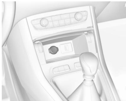
A 12 V power outlet is located behind the storage cover. Press cover to open.
