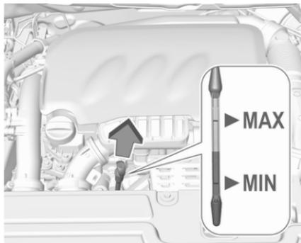
Pull out the dipstick, wipe it clean, reinsert it fully, pull out and read the engine oil level.
