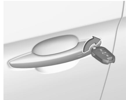
Manually lock the left front door by inserting and turning the key in the lock cylinder.
