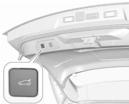
To close, press
