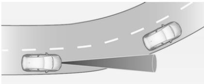
The adaptive cruise control calculates a predicted path based on the centrifugal force. This predicted path considers the current bend characteristic, but cannot consider a
