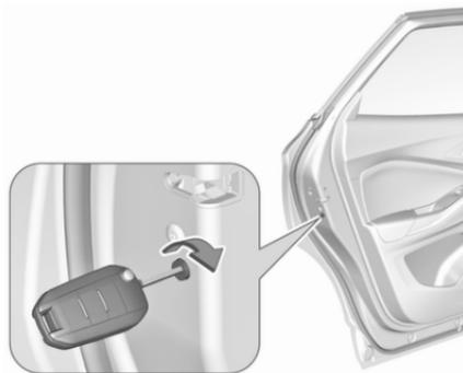
To lock the other doors, remove the black cover by using a key.
