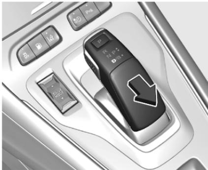
To activate **B**, select **D** and push the selector lever backwards. To shift out of **B**, push the selector backwards again.
