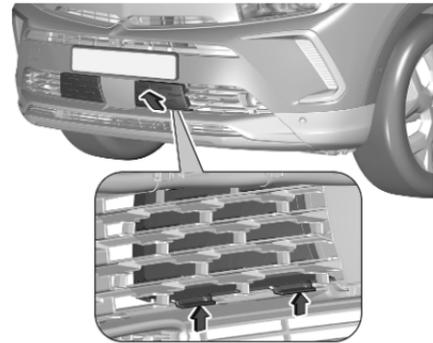
1. With your hand behind the grille, push the brackets of the protection covers upwards to release them.
