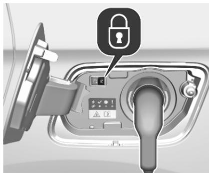
Once charging, the vehicle plug will be locked to the charging port and cannot be disconnected while charging is active.
