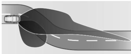
Particular LEDs, based on steering angle and speed, are additionally triggered to improve lighting in curves. This function is activated at a speed up to approx. 43 mph.
