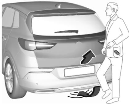
To open or close the tailgate, move the foot in the center area below the rear bumper back and forth quickly. Do not hold the foot under the bumper. The electronic key must be outside the vehicle, within a range of approx. 1 m of the tailgate. When foot motion is being detected by the sensor, the system actuates the tailgate after a short delay.
