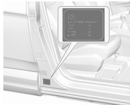
The identification plate is located on the front left or right door frame. The layout and position differ for some export countries.
