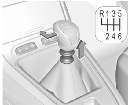
To engage the reverse gear on 6-speed transmission, with the vehicle stationary and engine at idle depress the clutch pedal, pull the ring under the selector lever and move the selector lever quite to the left and front.
