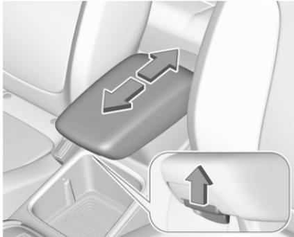
The armrest can be slid forwards by 10 cm. Pull the handle to slide the armrest. Under the armrest there is a storage compartment.
