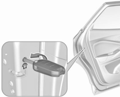
Turn the red child lock in the rear door to the horizontal position by using a key. The door cannot be opened from the inside.
