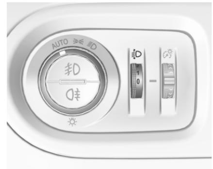
To adapt headlight range to the vehicle load to prevent dazzling, turn thumb wheel
