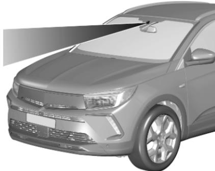
The activated system observes the lane markings by using the camera located at the top of the windscreen. It steers the vehicle inside the
