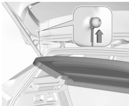
Unhook the retaining straps from the tailgate.
