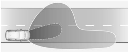
If bad weather conditions are detected, low beam is dimmed to avoid dazzling the oncoming traffic.
