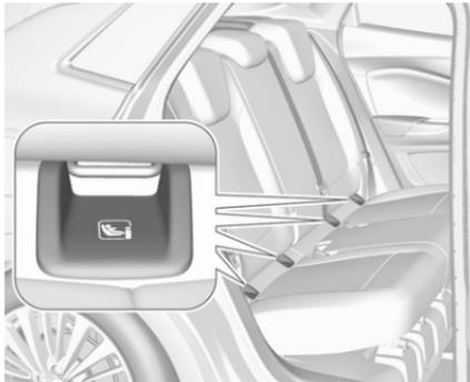
Fasten vehicle-approved ISOFIX child restraint systems to the ISOFIX brackets. Specific vehicle ISOFIX child restraint system positions are marked in the ISOFIX table ↻ 49.
