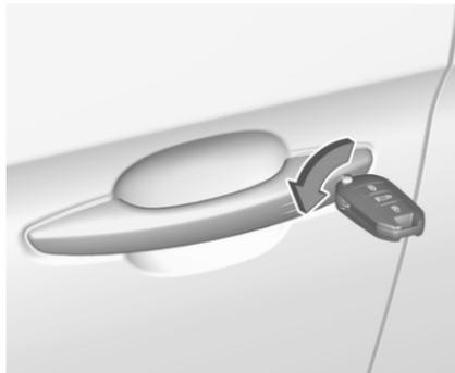
Manually unlock the left front door by inserting and turning the key in the lock cylinder.
