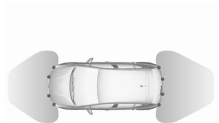
The system operates with ultrasonic parking sensors in the rear and front bumper.
