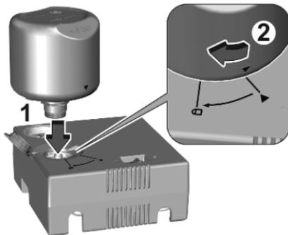
5. Type A: First, insert sealant bottle into the compressor and align the triangle symbols. Then, push down sealant bottle and turn it to the lock position.
