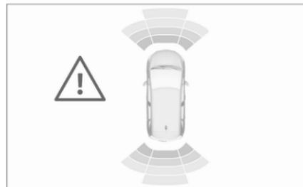
Additionally, the distance to rear and front obstacles is displayed by changing distance lines in the Info Display ↗ 85.
