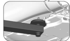
Rear arm position of the lifting platform centrally under the relevant vehicle jacking point.
