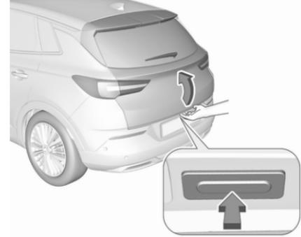
To open the tailgate, press the tailgate button until the tailgate starts to move. If the vehicle is locked, the electronic key must be outside the vehicle, within a range of approx. 1 m of the tailgate.
