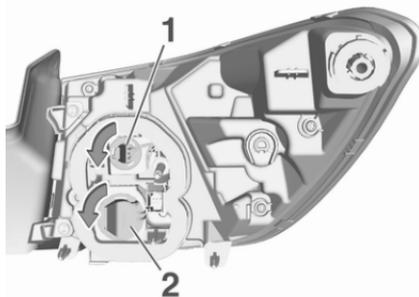
7. Detach the bulb from the bulb socket and replace the bulb.
