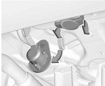
Disengage and fold down the socket. Remove the sealing plug from the opening for the coupling ball bar and stow it.
