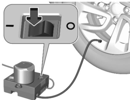
12. Set the rocker switch on the compressor to I. The tyre is filled with sealant.
