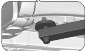
Front arm position of the lifting platform centrally under the relevant vehicle jacking point.
