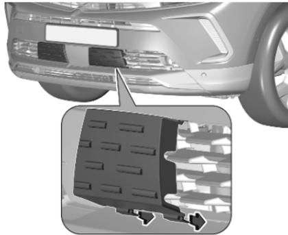
Press the lower part of the protection covers against the slat of the grille. Ensure that the protection covers are fixed securely.
