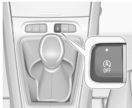
Deactivate the stop-start system manually by pressing
