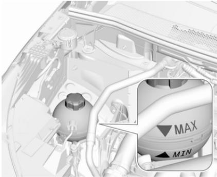
If the cooling system is cold, the coolant level should be above the **MIN** mark. Top up if the level is low.
