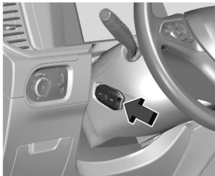
Hold the electronic key with buttons outside at the marking on the steering column cover as shown in the illustration.
