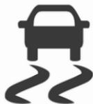
ESC and traction control system are operational after each engine start as soon as the control indicator
