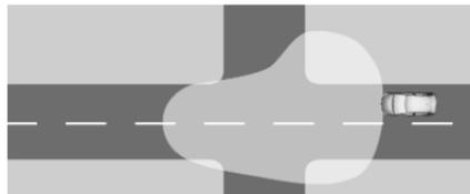
Activated automatically at a speed up to approx. 31 mph. The beam has a broad shape to avoid glaring oncoming traffic.
