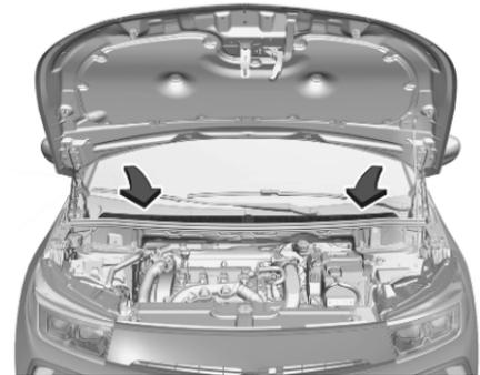
The air intake in front of the windscreen in the engine compartment must be kept clear to allow air intake. Remove any leaves, dirt or snow.
