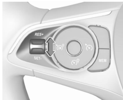
Accelerate to the desired speed and move thumb wheel once briefly to **SET/-**. The current speed is stored as maximum speed.
