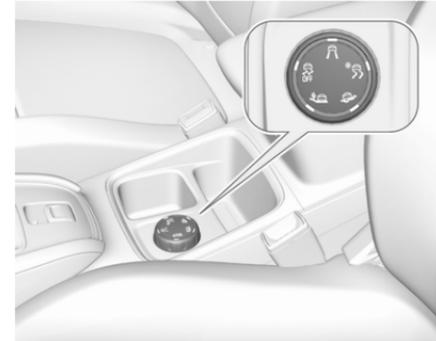
Selective ride control allows to choose between five driving modes by turning the control:
