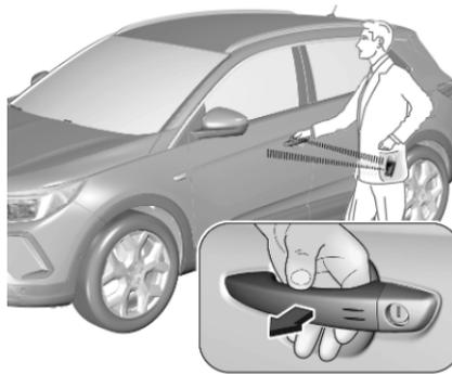
The electronic key must be outside the vehicle, within a range of approx. 1 m of the relevant door side.
