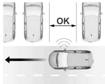
When a free slot is detected, a visual feedback on the Info Display and a first acoustic signal are given. Drive slowly forwards. When the second acoustic signal is given, stop the vehicle, select reverse gear, release the steering wheel and start moving slowly. A visual feedback is given on the Info Display.
