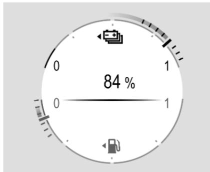
The battery gauge displays the high voltage battery state of charge.
