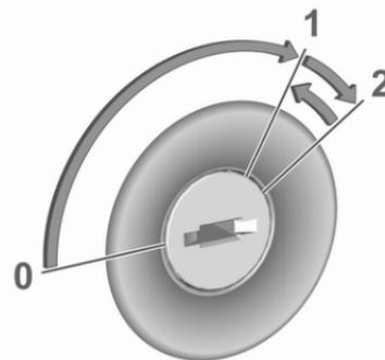
Turn key to position 1 to release the steering wheel lock.
