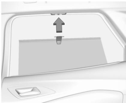
To reduce sunlight at the second row seats, pull the blind upwards using the grip and engage it at the top of the door frame.
