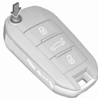
Press button to extend. To fold the key, first press the button.
