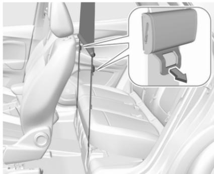
Pull the flap at the tightener on both sides to release the straps. Detach hooks from the lashing eyes.
