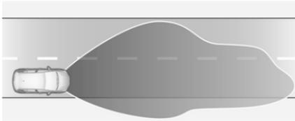
Activated automatically at a speed above 30 mph when driving in rural areas. The illumination of the current lane and the side of the road is adapted. Oncoming and preceding vehicles are not dazzled.
