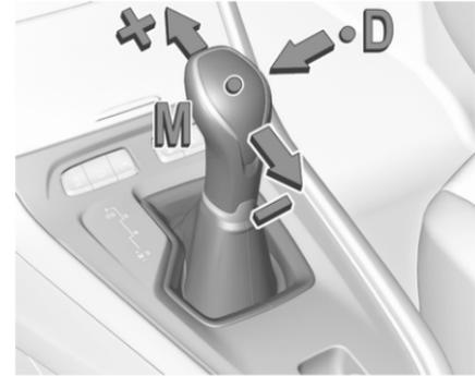
Move selector lever out of position **D** towards the left in position **M**.
