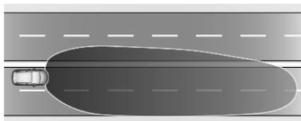
Activated automatically at a speed above 65 mph. Illumination is adapted to the higher speed driven on motorways. If there is no oncoming traffic, the visibility on the side of the vehicle is increased. When following vehicles ahead or passing, dazzling for these vehicles is reduced.
