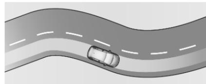
Thus, the current position of the vehicle within the lane is kept. This position is not necessarily the centre of the lane.
