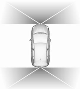
The 180° view facilitates reversing out of a parking bay, making it possible to see the approach of vehicles, pedestrians and cyclists. This view is not recommended for carrying out a complete manoeuvre. It is made up of three areas: left 1, centre 2 and right 3. This view is available from the view selection menu only.
