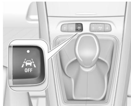
If the system is activated, the LED in the button
