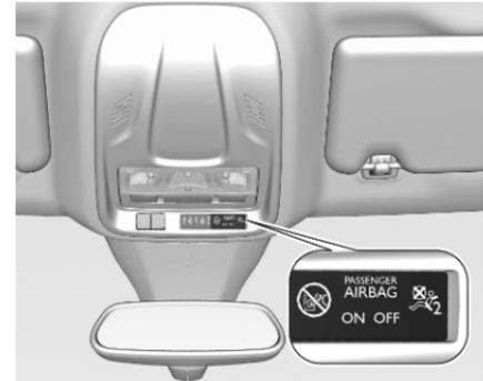
If the control indicator
