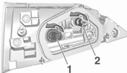
6. Turn the bulb socket anticlockwise and remove it from the light assembly.
