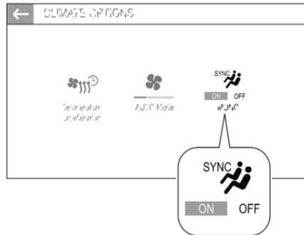
Set **SYNC** to **ON** to link passenger side temperature setting to the driver side
