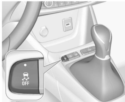
ESC and traction control system can be deactivated if it is required: press
