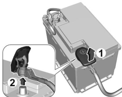
9. Lift the plastic cover of the vehicle battery's positive terminal in the engine compartment.
