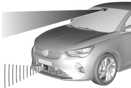
The forward collision alert uses the front camera in the windscreen and depending on the vehicle configuration a radar unit located behind the front bumper to detect a vehicle directly ahead, in the path.
