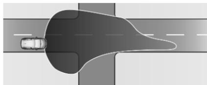
Activated automatically at a speed up to approx. 30 mph. The light is wide and symmetrical.
