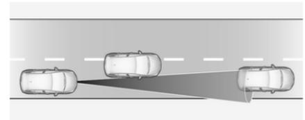
If another vehicle enters your driving path, adaptive cruise control will first consider the vehicle when it is completely in your path. Be ready to take action and depress the brake pedal if you need to brake more quickly.
