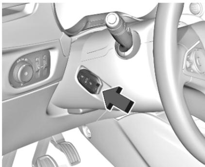
Hold the electronic key at the marking on the steering column cover as shown in the illustration.
