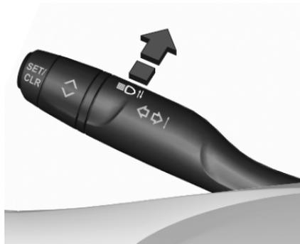
Push to switch from low to high beam.
