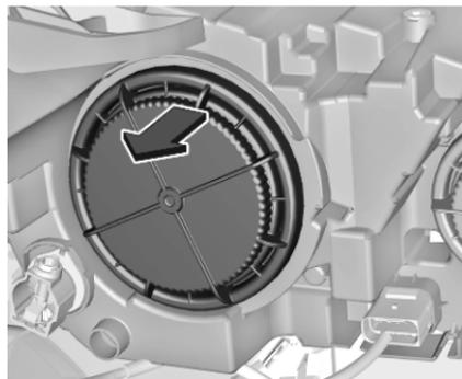
1. Remove the protective cover by pulling.
