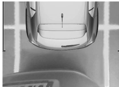
The camera records the vehicle's surroundings during the manoeuvre in order to reconstruct a view from above the rear or the front of the vehicle in its near surroundings. Thus, the vehicle can be manoeuvred
