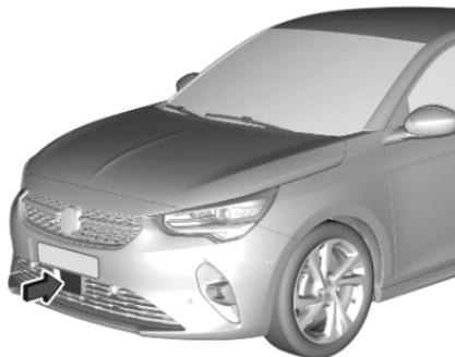
The radar unit is located in the middle of the front bumper.
