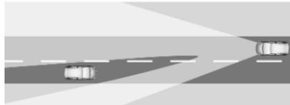
Each LED on right or left side is triggered or faded out particularly according to the traffic situation. This gives the best light distribution without dazzling other road users.
