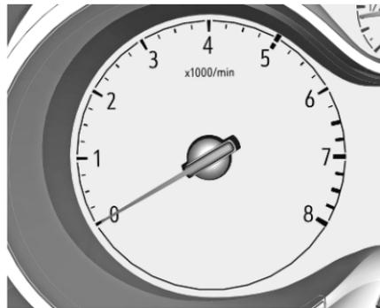
Displays the engine speed.
