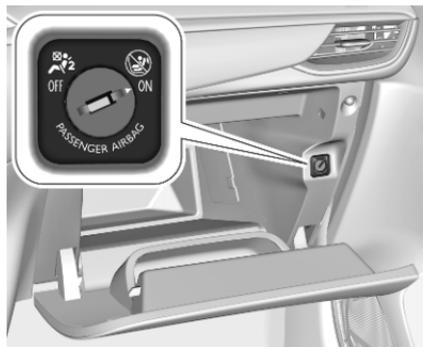
The front passenger airbag system can be deactivated via a key-operated switch in the glovebox.
