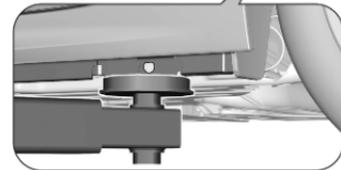
Rear arm position of the lifting platform centrally under the relevant vehicle jacking point.
