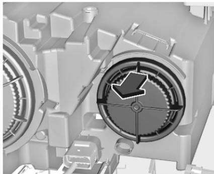
1. Remove the protective cover by pulling.
