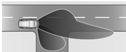
Activated at a speed of up to 25 mph when turning off. The light consists of particular LEDs which illuminate the direction of travel. These LEDs are
