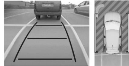
The screen in the Info display is divided into two parts. On the right there is a view from above the vehicle, and on the left there is the view from the rear displayed. The parking sensors complete the information on the view from above the vehicle.
