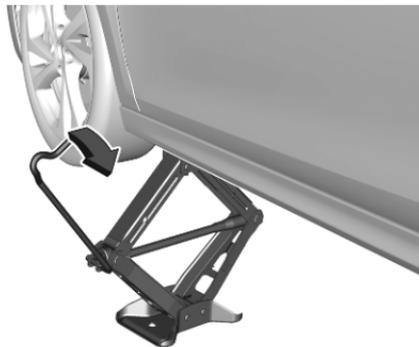
With the jack correctly aligned rotate wheel wrench until wheel is clear of the ground.
