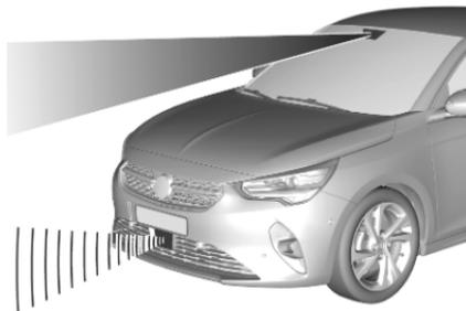
The system uses the front camera in the windscreen and depending on the vehicle configuration a radar unit in the front bumper to detect a pedestrian directly ahead in the path.
