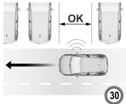
When a free slot is detected, a visual feedback on the Info Display and an acoustic signal are given. Stop the vehicle, select reverse gear, release the steering wheel and start moving without exceeding 4 mph.
