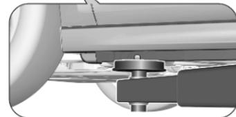
Front arm position of the lifting platform centrally under the relevant vehicle jacking point.
