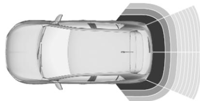
Additionally, the distance to rear obstacles is displayed by changing distance lines in the Info Display  $\rightarrow$  74. When the obstacle is very close,  $\triangle$  for danger is displayed.
