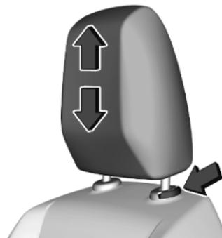
Pull the head restraint upwards or press the catch to release and push the head restraint downwards.
