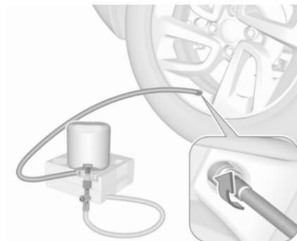
7. Screw the filler hose to the tyre valve.
