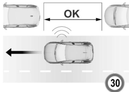
When a free slot is detected, a visual feedback on the Info Display and a first acoustic signal are given. Drive slowly forwards. When the second acoustic signal is given, stop the vehicle, select reverse gear, release the steering wheel and start moving slowly. A visual feedback is given on the Info Display.
