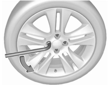
2. Attach the wheel wrench and loosen each wheel bolt by half a turn.
