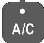
Press **A/C** to switch on cooling. The LED in the button illuminates to indicate activation. Cooling is only functional when the engine is running and fan is switched on.
