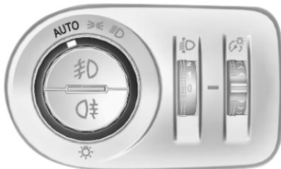
When the automatic light control function is switched on and the engine is running, the system switches between daytime running lights and headlights automatically depending on the external lighting conditions and information given by the wiper system.
