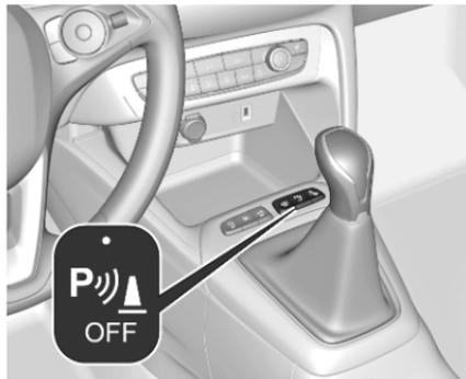
The system is switched off when reverse gear is disengaged. Press  $P_{OFF}$  to deactivate the system manually. The LED in the button illuminates when the system is deactivated. If the system has been deactivated manually, it is not reactivated automatically the next time the ignition is switched on.
