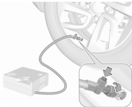
16. Continue driving immediately so that sealant is evenly distributed in the tyre. Drive between 13 mph and 37 mph. After driving approx. 3 miles but no more than 10 minutes, stop and check tyre pressure. Screw compressor air hose directly onto tyre valve when doing this. Fill tyre as described before. Drain excess tyre pressure with the button on the air hose.
