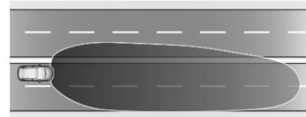
Activated automatically at a speed above 65 mph. Illumination is adapted to the higher speed driven on motorways. If there is no oncoming traffic, the visibility on the side of the vehicle is increased. When following vehicles ahead or passing, dazzling for these vehicles is reduced.
