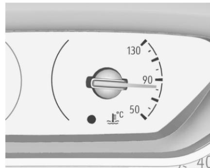
Displays the coolant temperature.
