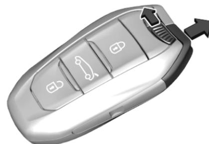
Electronic key: push the latch to extract the integral key.
