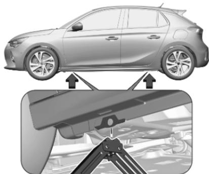
3. Ensure the jack is correctly positioned under the relevant vehicle jacking point.
