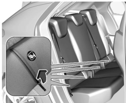
Fasten vehicle-approved ISOFIX child restraint systems to the ISOFIX brackets. Specific vehicle ISOFIX child restraint system positions are marked in the ISOFIX table ⇨ 43.
