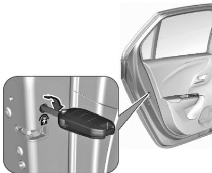
Turn the red child lock in the rear door inwards to the horizontal position by using a key. The door cannot be opened from the inside.
