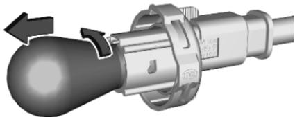
2. Slightly press down the bulb, turn it anticlockwise and remove it from the socket.
