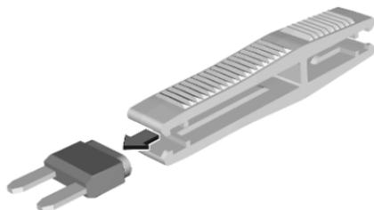
Grab the fuse with the fuse extractor and withdraw the fuse.
