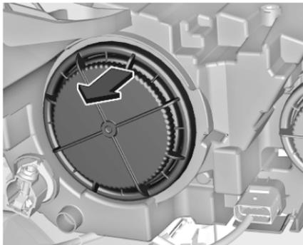
1. Remove the protective cover by pulling.
