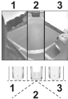
The 180° view facilitates reversing out of a parking bay, making it possible to see the approach of vehicles, pedestrians and cyclists. This view is not recommended for carrying out a complete manoeuvre. It is made up of three areas: left 1, centre 2 and right 3. This view is available from the view selection menu only.
