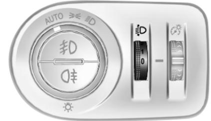
To adapt headlight range to the vehicle load to prevent dazzling, turn thumb wheel
