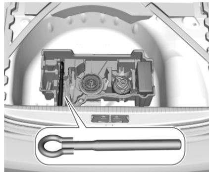
The towing eye is located in a box below the floor cover in the load compartment.
