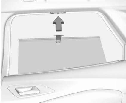
To reduce sunlight at the rear seats, pull the blind upwards using the grip and engage it at the top of the door frame.
