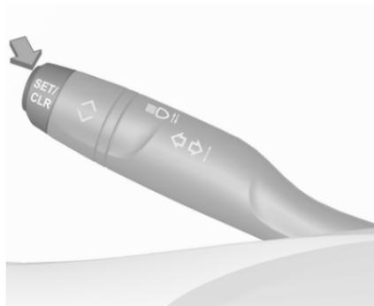
Press **SET / CLR** for 2 seconds to reset the trip odometer.
