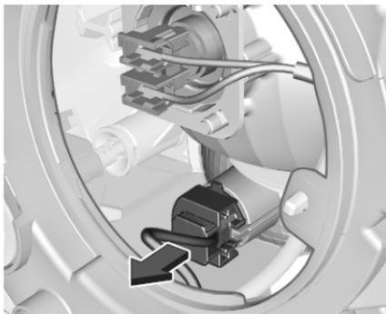
2. Withdraw the bulb socket from the reflector housing.
