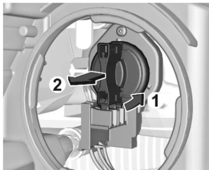
2. Rotate the bulb socket anticlockwise to disengage and withdraw from the reflector.
