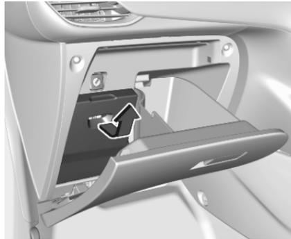
In right-hand drive vehicles, the fuse box is located behind a cover in the glovebox. Open the glovebox and remove the cover.
