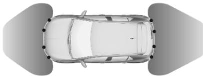
The system operates with ultrasonic parking sensors in the rear and front bumper.
