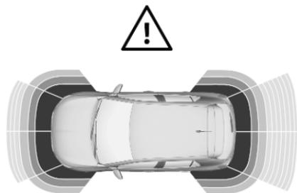
Additionally, the distance to rear and front obstacles is displayed by changing distance lines in the Info Display ↗ 74.
