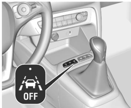
If the system is activated, the LED in the button
