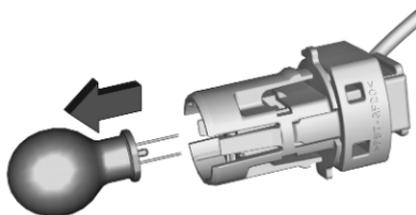
3. Detach the bulb from the bulb socket and replace the bulb.
