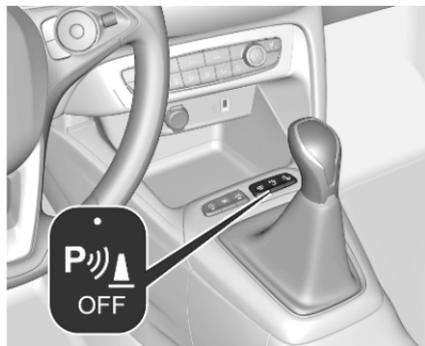
The system is ready to operate when the LED in the parking assist button  $P_{OFF}$  is not illuminated. The state of the system is memorised when the ignition is switched off.
