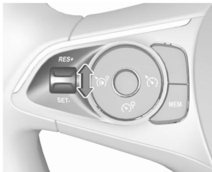
Accelerate to the desired speed and move thumb wheel once briefly to **SET/-**. The current speed is stored and maintained. Accelerator pedal can be released.
