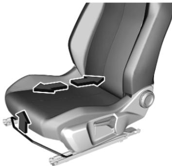
Pull handle, slide seat, release handle. Try to move the seat back and forth to ensure that the seat is locked in place.
