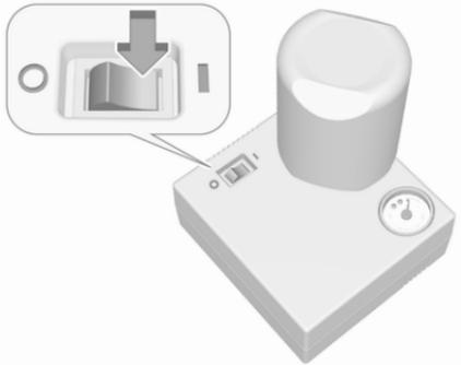
10. Set the rocker switch on the compressor to I. The tyre is filled with sealant.
