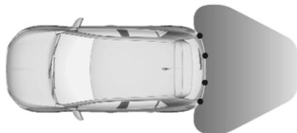
The system operates with ultrasonic parking sensors in the rear bumper.
