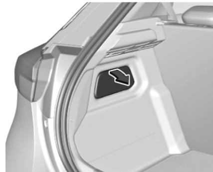
1. Open the tailgate then remove the access cover on the relevant side.
