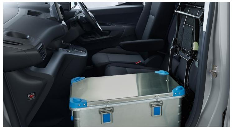
Load-through hatch within bulkhead.
