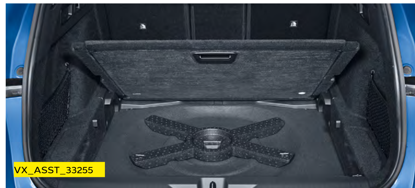
Intelli-Space adjustable load floor.
