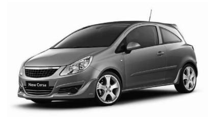
Model illustrated features Irmscher front lower spoiler, side sills, cross hatch grille – black with aluminium upper and laser-etched 'Irmscher' logo, rear hood spoiler and 17-inch Sport Star alloy wheels.
