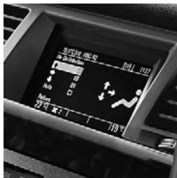
Electronic Climate Control (ECC) display as featured on Vectra.
